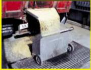
this photo. It mounts on a couple wheels and is fitted with a handle across the top, making it easy to roll into position under the endgate. Made from plywood, it's simply a box that's higher in the back than the front, helping direct flow of grain down through the grates. (Dave White, 32202 E. Second Rd., Farmersville, III. ph 217 227-3659)
