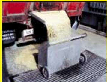
this photo. It mounts on a couple wheels and is fitted with a handle across the top, making it easy to roll into position under the endgate. Made from plywood, it's simply a box that's higher in the back than the front, helping direct flow of grain down through the gates. (**Dave White, 32202 E. Second Rd., Farmersville, Ill. ph 217 227-3659**)
