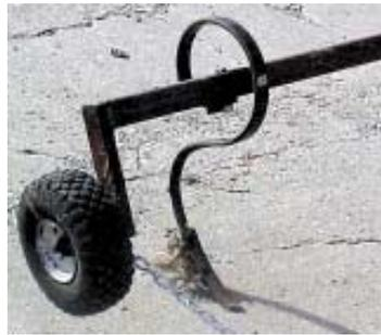
Marker unit consists of a shank attached to a length of sq. tubing. A small wheel serves as a depth gauge. Chain runs from end of marker to pickup's front bumper.
