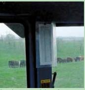
Chart in tractor cab is used to convert pounds of pressure to pounds of hay.
