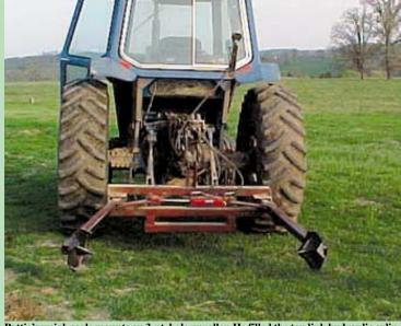
Pattie's weigh scale mounts on 3-pt. bale unroller. He filled the top link hydraulic cylinder with fluid and then ran a hose into a 600 psi pressure gauge. Bale exerts pressure on top link, which affects pressure reading.
