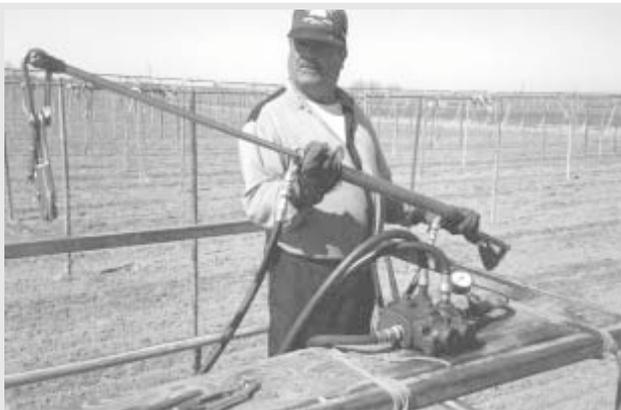
Stretcher has a 1 1/2-in. dia. cylinder with a 3/4-in. dia. rod and a come-along pinned to each end. Cylinder is controlled by open center valve equipped with a pressure gauge.
