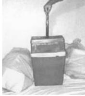
When basket gets full, you just pull out and up on a push rod and then push down to crush trash with a plunger built into lid.
