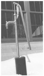
Pump operates without electricy and installs on top of any existing well casing that extends above ground.
