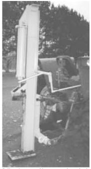
Splitter is operated by a remote lever that's connected by linkage to tractor's hydraulic lever. Hook welded onto drawbar mounting bracket lets Switzer use a "logger's choker" to skid trees.
