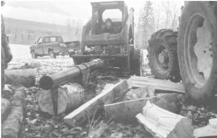
Splitter consists of a 6-in. dia., 8-ft. long, heavy-walled steel pipe with a fixed wedge at one end. Push plate slides back and forth on the pipe.
