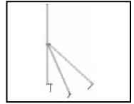
Tripod corner post has a solid steel spike which can be stepped in or driven into ground. Free-swinging braces are attached about half way up the post.
