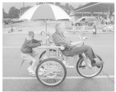
Funk's home-built 3-wheel cycle has a seat on back for a small passenger and an extra set of pedals. "My 6-year-old grandson Charlie does most of the pedaling," says Funk.
