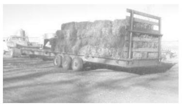
Jim Cook, Zearing, Iowa, used the frame and axles off an old mobile home to build his high-capacity hay hauler. He uses a Chevy 1-ton dually pickup to pull it.
