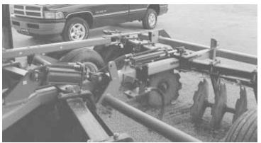
"It lets me adjust the angle of disk's rear gangs automatically on-the-go," says Glenn Buck about the hydraulic-powered conversion he made on his 14 1/2-ft. disk.
