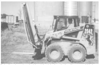
Bale slicer is equipped with a 6-ft. 10-in. long hydraulic-operated blade.
