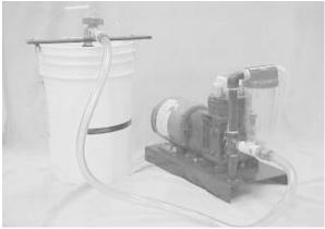
Pump primer consists of an electric motor and an air conditioning compressor that generates 20 to 25 lbs. of suction, along with a clear plastic bulb and a valve. Photo shows pump pulling water out of bucket.
