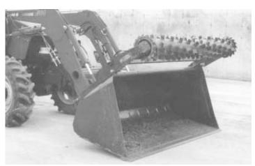
Valmetal rotary silage cutter is designed to remove hard-packed silage from bunker silos. Arms weld onto bucket of any front-end loader, skid loader, or payloader.
