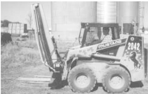
**Bale slicer is equipped with a 6-ft. 10-in. long hydraulic-operated blade.**
