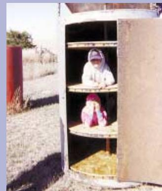
Built out of a 500-gal. fuel tank, tool cabinet contains four rotating “Lazy Susan”-type shelves.
