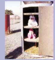
Built out of a 500-gal. fuel tank, tool cabinet contains four rotating "Lazy Susan"-type shelves.
