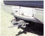
Hitch assembly consists of ball hitch and straight drawbar. Note small ball on bumper.
