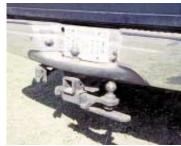
Hitches are carried out of the way, underneath the back edge of bumper.
