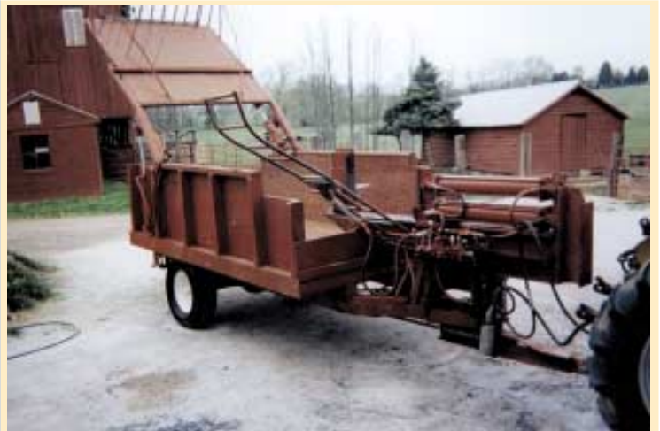
Two-wheeled machine has a log loading ramp on front and a 15-ft. trailer on back that's dumped by a 5-ton wagon hoist. Rear tailgate also loads wagon box with wood.
