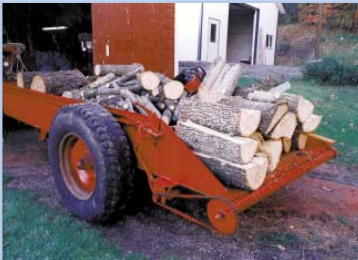
Two-wheeled trailer is built on chassis of an old manure spreader. Wood is pulled to the back by a pair of stainless steel cables that wrap around a drum at back of trailer.
