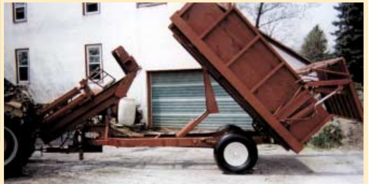
Wood is unloaded out the back by raising splitter unit up out of the way, then opening the tailgate and raising the trailer.
