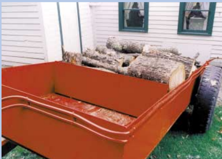
An L-shaped metal plate, with nylon skid shoes under it, moves from front of trailer to back to push off the load.
