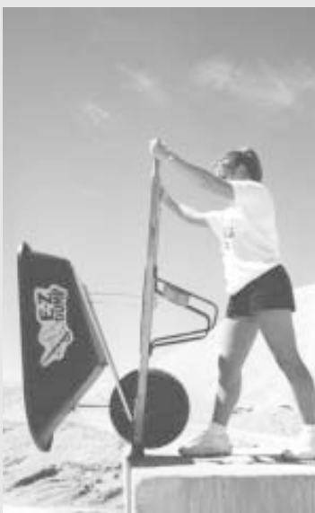
Bolt-on kit causes cart to pitch forward off the handles and dump its load as you raise wheelbarrow handles.
