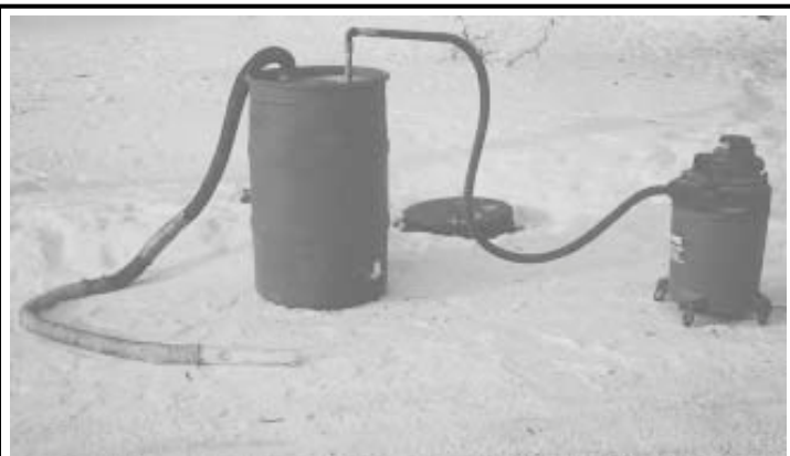
"It lets me vacuum up a barrel full of liquid at a time," says Glen Woodside, who connected a 55-gal. plastic barrel to a shop vac.
