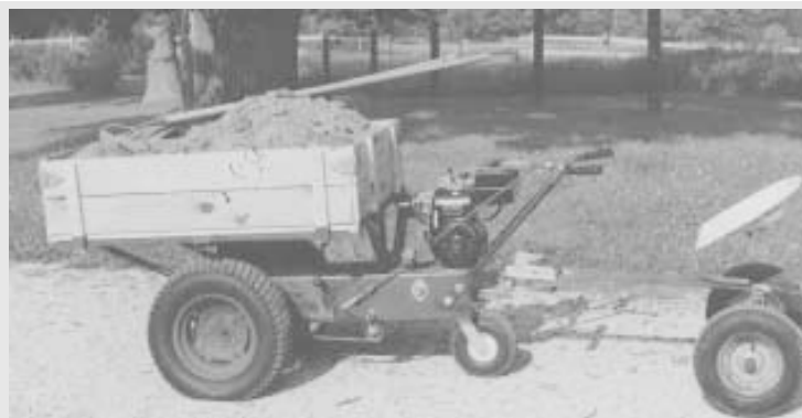
Starting with a junked 12 hp Sears lawn tractor, Ron Mickle built this self-propelled wheelbarrow. The rear wheels bear the load and power the wheelbarrow.
