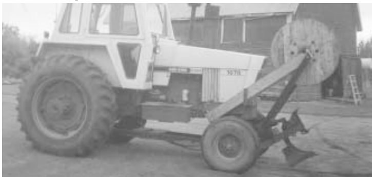
Lesiuk turned an old moldboard plow beam into a trencher. It fits on dozer mounts at the front of his Case 1070 tractor.
