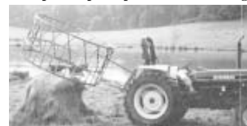
Bracket is available in two different sizes of receiver tubes to fit different bale spears.
