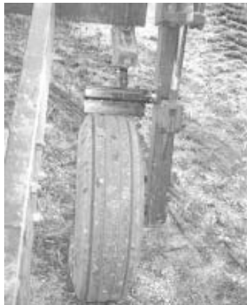
Adjustable scraper attaches to cultivator toolbar with a simple bolt-on bracket.
