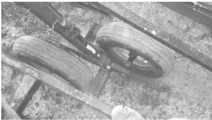
Legner made scrapers to keep the wheels clean on his Case-IH 4600 field cultivator.
