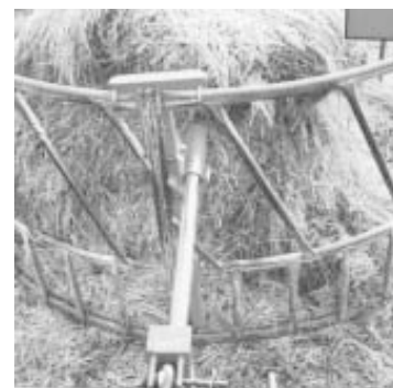
Feeder-mounted bracket lets you use a bale spear to pick up and move bale ring.
