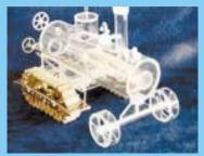
This is a model of the first tractor ever made with tracks, invented in 1893 by Charles Stratton. The tractor steered with its front wheels. Note the two steering control wheels - one for each track.
