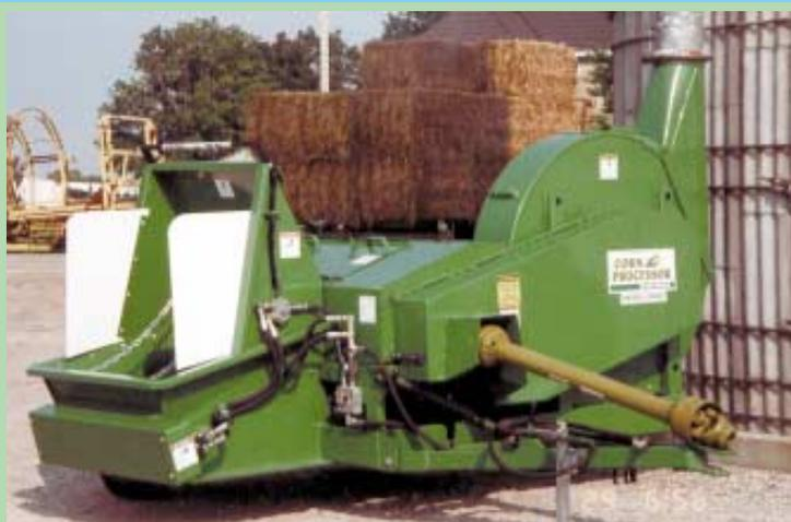
**Silage goes in one side and is forced through a roller mill before being sent through the blower fan and up the tube into silo.**
