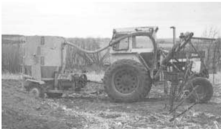
Pto-powered feed grinder blows a mixture of oats and brome through a hose up to a 20-ft. long, tractor-mounted boom that’s hydraulically raised or lowered.
