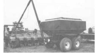
Tandem axle seed loading unit is complete with a hydraulically-operated auger and 15-ft. telescoping downspout.
