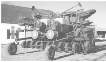
Nieman built his 16-row, 16-in. soybean planter (above) out of two used IH 500 Cyclo air planters. He added Keeton seed firmers to Acra-Plant shoes (right) to keep seed from bouncing out of the ground. mounting brackets interfered with the hinge where the toolbar folds on each side so I just went 1 inch wider."
