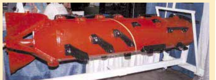
"High-inertia" rotor is actually a rebuilt Case-IH rotor. Kuchar re-attaches the rub bars in a more open design which allows the crop to go through faster without "slugging down" the rotor.
