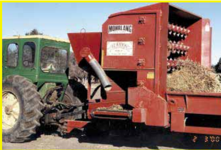
Conveyor belts move bales forward into flail cutters that pull hay and straw off bale ends. Another conveyor drops material into a bunk or on the ground.
