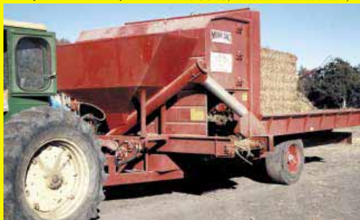
Hopper attachment on front of processor allows grain or pelleted feed to be mixed into the hay as it drops into the feed bunk.
