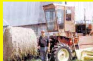
for the combine which is equipped with tilting bale forks on front. The bale forks are operated by an extra hydraulic valve that runs off the combine's hydraulic pump which used to operate the header. It can load bales one high on a trailer. **(Thomas Biver, 24684 King Road, Spooner, Wis. 54801 ph 715 635-2851)**
