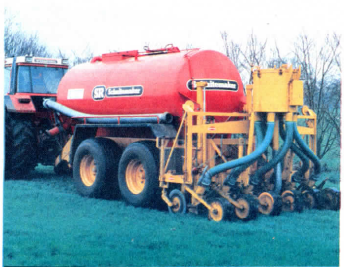
Manure flows from rear-mounted distribution tank to injection tines mounted behind coulters. Tines create furrows that are closed by a pair of spring-loaded press wheels.
