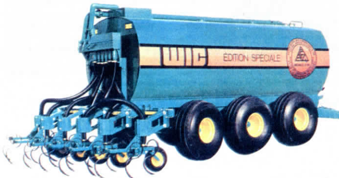
Front and rear axles are connected by closed circuit hydraulic system that allows giant spreader to turn on corners and headlands without damaging crop.
