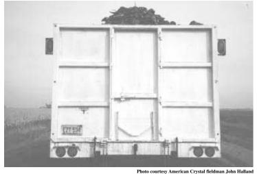
Mud from rear wheels often covered the tail lights on Barry Malme's truck. To solve the problem he mounted an extra pair of tail lights 5 ft. up from the original ones.
