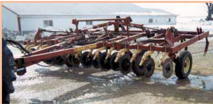
Using his 12-ft. Sunflower chisel plow as a base, DeShaw built a 17 1/2-ft. folding, self-leveling plow.
