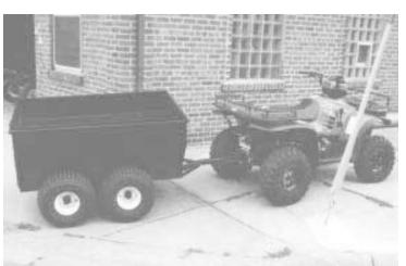
Tandem axle suspension gives ATV trailer plenty of carrying capacity for farm chores.
