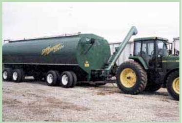
"Grain Station 2000" measures 12 ft. wide and 36 1/2 ft. long. Fully loaded, it holds 61 tons and has 50 percent more capacity than a conventional semi truck.
