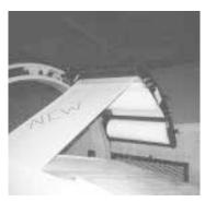
Two rolls of plastic are unrolled at once. As they're pulled, they bond tightly together forming a laminated double layer of plastic that's much more resistant to puncturing, says Horst Welding.
