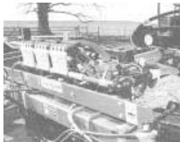
System makes use of a Red Ball monitor which consists of clear plastic tubes with balls floating in them. They tell you at a glance how each row is operating.
