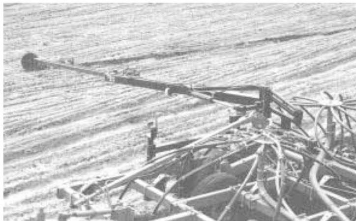
Marker mounts on rear corner of air seeders and cultivators. It swings forward and telescopes to the desired length and leaves a groove of about 2 in. in the ground.
