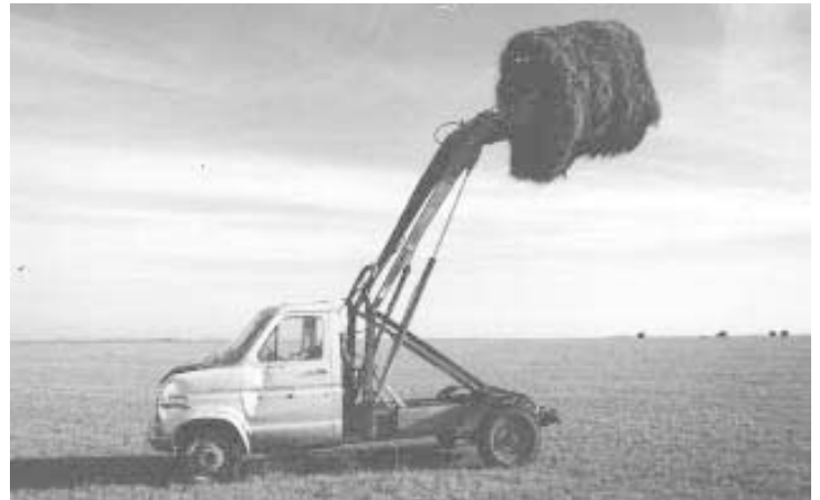
Maxfield stripped off the back of a Ford van and fitted it with a Farmhand F11 loader.
