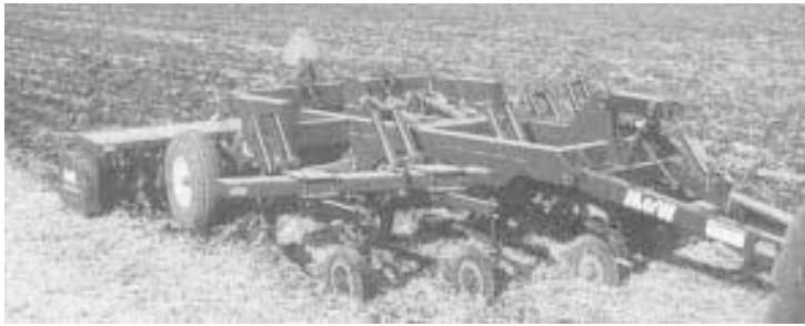
“Dyna-Master” lets you subsoil and finish fields in a single pass, reducing compaction and maintaining residue at the same time.
