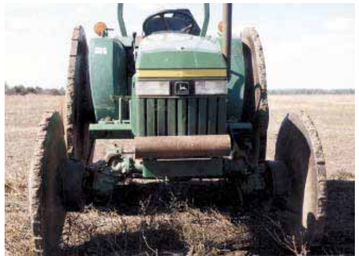
Homemade steel wheels measure 5 ft. high on back and 3 ft. high on front. Wheels make V-shaped, 4 to 6-in. deep ditches that drain water out of fields.
