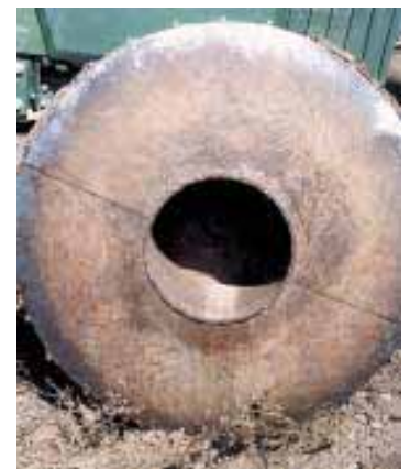
A 10-in. dia. steel pipe serves as the hub for each wheel. Easley used 3/8-in. thick reinforced steel plate to make the wheels.
