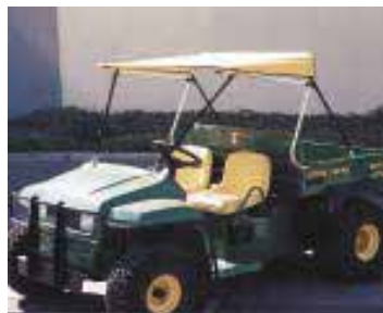
"Bimini Top" is made from marine grade vinyl supported by a lightweight aluminum frame.
