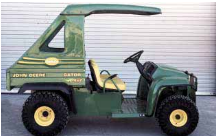
Bed-mounted canopy designed for the Gator 4 by 2 is made from lightweight, rigid fiberglass. No drilling of holes is required.
