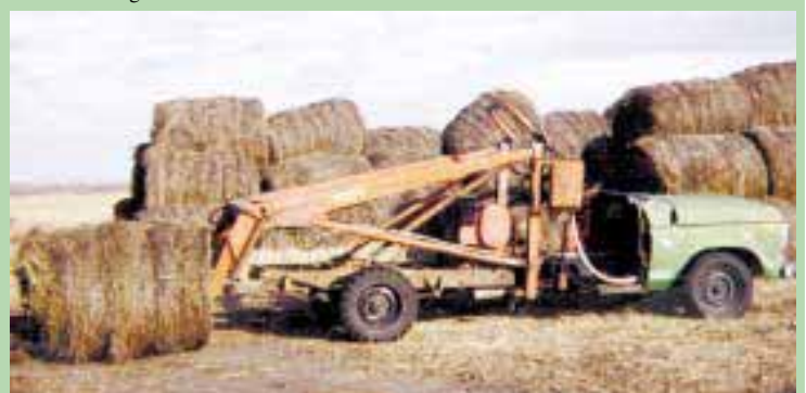
To help support weight of bale, Sullivan replaced pickup's original rear wheels with 10.00 by 16.5 skid steer tires. He can stack bales up to four high.
