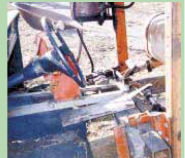
To operate the loader, he sits on a seat next to the steering wheel that faces backward, and runs the transmission in reverse.
