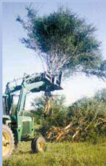
Brush puller mounts on front-end loaders with a 3,000-lb. lift capability, or a tractor 3-pt. hitch. It can uproot an 8-in. Cedar tree 25 ft. tall.
