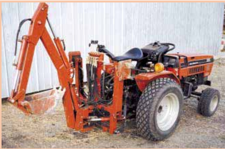
Brown's 3-pt. hitch backhoe attachment fits his Case-IH 235 18 hp diesel tractor.
