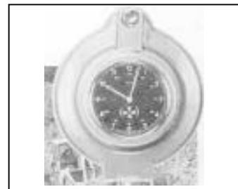
Recorder helps with preventative maintenance by telling you how many hours the engine has actually been working as opposed to idling.
