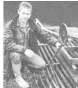
Wright fitted a 9-in. dia. ballcock on a rod attached to a pivot point. Ballcock rises as slurry nears the top, raising "lollipop-shaped" disc into the air.
