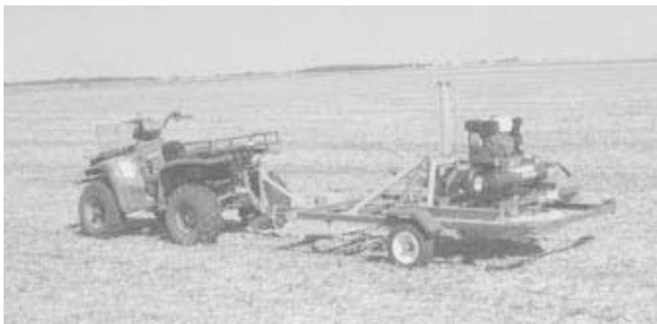
“Air Probe” mounts on a 2-wheeled trailer and is equipped with a large turntable that holds 20 small containers. Power is supplied by a small air compressor.
