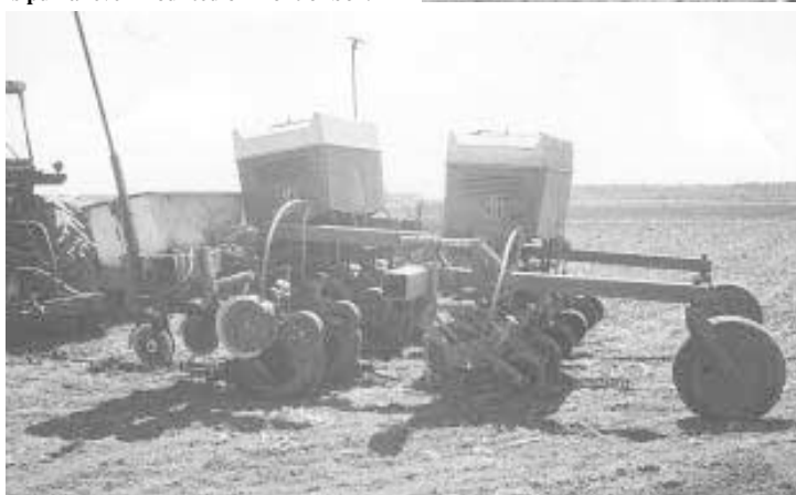
Wallace's twin-row planter is built out of two Case-IH 800 6-row air planters. It plants six sets of twin rows spaced 8 in. apart, with 22 in. between each set of rows.
