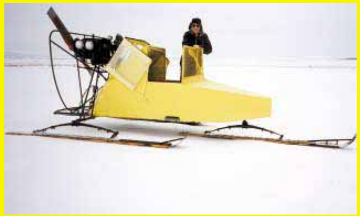
Air-powered "snow plane" is powered by a big airplane propeller and rides on three 9-ft. long aluminum skis. "It's a lot of fun to drive," says Weimerskirch.
