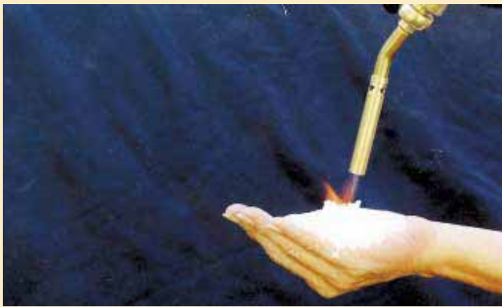
Ceramic powder can be mixed into any paint. The fine white powder was developed by NASA for the space shuttle. Photo shows how it dissipates heat.
