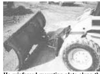
He reinforced mounting plate along the edges and across the center by welding channel iron on back.
