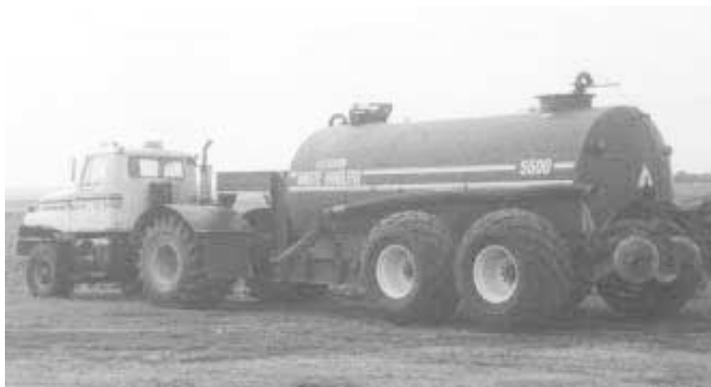
"It lets us go fast and reduces compaction," says Dennis Hess, who converted a "Terra Truck" floater sprayer to pull a big liquid manure tank equipped with injectors.
