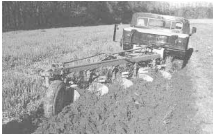
Tom Kendle thinks Hummers make perfect farm utility vehicles, especially when equipped with his 3-pt. hitch and pto. Here he's using it to pull a five-bottom plow.
