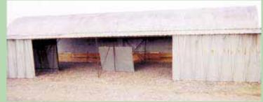
Miller used some of the pie-shaped roof panels to make partial walls along the open side of the building.
