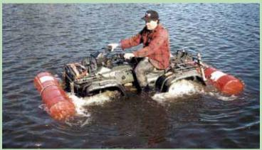
A length of pipe clamps onto exhaust muffler to serve as a "snorkel". Another snorkel fits the air intake (not shown). The snorkel allows water to wash over ATV.
