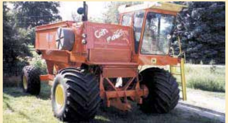
Henning left the cab and engine in place and fitted the self-propelled grain cart with flotation tires. It'll carry 600 bu. at full speed across fields.
