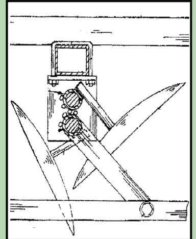
Drawing shows how variable discs are rotated on front of tillage tools.
