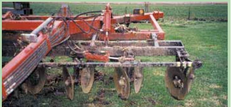
Discs can be angled anywhere from 0 to 38°, depending on conditions. Soil is mixed between discs, resulting in "vertical mulching" of residue that goes down much deeper than other methods.
