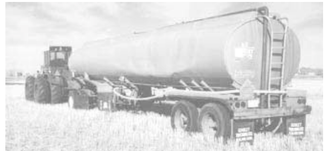
Water is delivered by an 8 hp gas engine and a pump mounted under tank.
