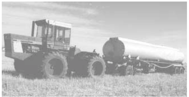
The 7,000-gal. semi tank mounts on a used converter dolly that has a drawbar hitch on front of it. Kirby uses his 4-WD tractor to pull the unit.
