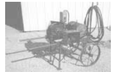
Two-wheeled unit is equipped with a 5 hp electric motor and a 3-speed transmission off an old pickup.
