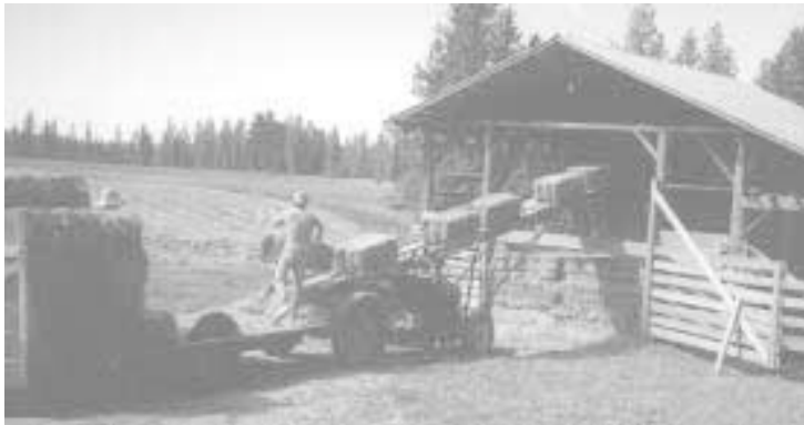
Machine works great for loading bales into sheds. The elevator can reach 16 ft. high.
