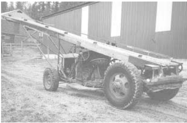
Skok built his self-propelled small square bale elevator out of a Dodge pickup and the rear axle and tires from a 2 1/2-ton Army truck.
