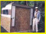
one of my ideas. It's a way to make use of an old pickup topper. I used it as a roof for a tool shed that stands in the back yard. The sides are made from particle board. I put a hinged door in the wood on one end. Many of the old toppers don't fit newer trucks so there are a lot of them around. (Bill Miller, Box 151, Landis, Sask. S2K 2KO Canada)
