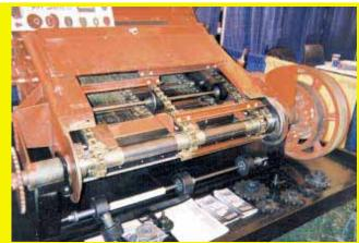
We recently introduced three feeder chain roller kits for all 60 and 80 Series Case-IH combines. The kits are designed to reduce wear on the feederhouse chain by keeping the chain off the upper and lower wear plates, which dramatically improves chain life and also makes it run quieter. Each kit includes a shaft, rollers, washers and nuts as needed for installation, as well as instructions and a template for drill-
