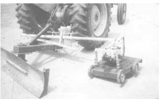
Hitch mounts on back of Strong's utility tractor and supports a 21-in. mower that swivels on the end of a 7-ft. long telescoping steel pipe.
