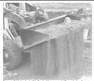
Bottom of "shaker bucket" is fitted with a screen. A 15 gpm hydraulic motor vibrates the entire bucket.
