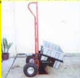
nuts. You dump the basket by pulling a latch and lifting up on a handle attached to the basket. By removing the wing nuts you can quickly remove the basket and use the handcart conventionally.
