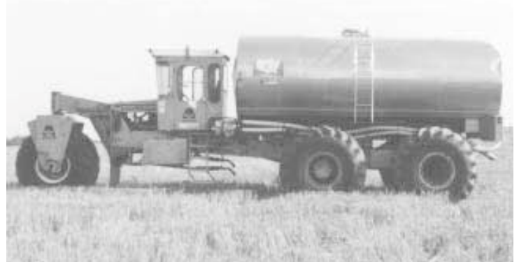
Weers mounted a 3,500-gal. stainless steel milk truck tank on a Big A 3-wheeled chemical applicator. An extra axle on back allows rear wheels to handle rough terrain.
