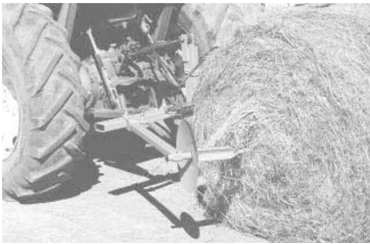
MacGregor's 3-pt. bale unroller is equipped with two pivoting side arms that are opened and closed by a hydraulic cylinder.
