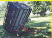
ran over it with a vacuum cleaner. The only time he has to get off the mower is when he's ready to dump the load. He simply unhooks the hose and opens the tailgate.
