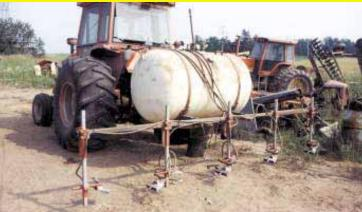
I'm trying to completely eliminate the use of chemicals on my farm, so I bought a commercial kit to build my own 3-pt. mounted, 6-row flame weed cultivator. The kit that I bought included the burners, burner mounting brackets, hoses, and controls. The company also offered an LP tank and a steel frame to support it, as well as the toolbar on which the burners mount but they wanted more than \$2,000 for those components. I
