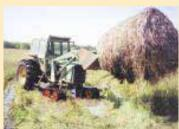
The 16-in. wide tracks can be used to replace the front wheels on 2-WD tractors.
