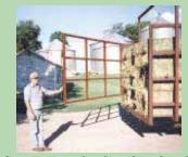
Operator can swing the endgate free allowing the stacked bales to slide free of the wagon when the hoist is engaged.
