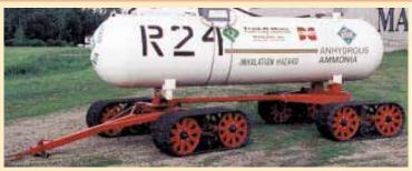
New "Trail-R-Mate" tracks are designed to mount on non-powered implements, such as this anhydrous ammonia running gear.
