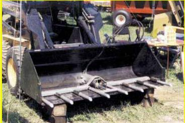
A set of 8-in. long retractable steel teeth mount inside bucket to tear silage loose. A single hydraulic cylinder extends or retracts the teeth.
